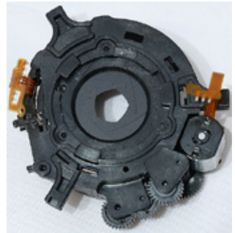
Aperture Mount from Canon 50mm f/1.8 lens
